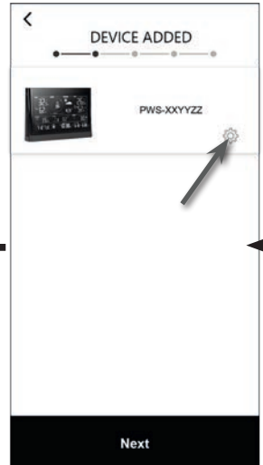
(d) Once the console is added to WSLink, the console icon will appear on your device list. Tap it to continue the setup.
